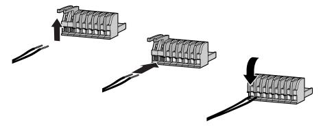
Figure 8. Inserting Wires into Terminal Blocks
